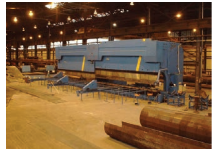
Figure 6. In the manufacturing (cold bending) of a polygonal section, tubular pole sections are fabricated by press-forming high-strength steel plate using a press brake.
